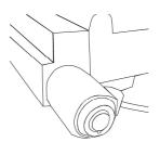
Lock the security cable in place using the keys provided.
